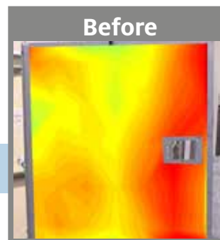
Before Vibration response test for truck utility door with welded vertical steel hat section. Red/yellow indicates high levels of vibration.
