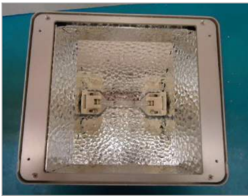
Figure 10. Reflector Housing with Glass Shield Installed
