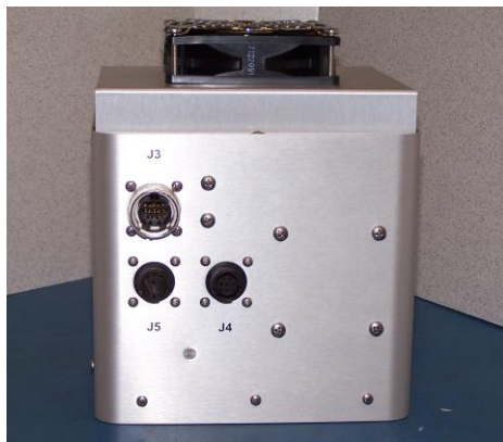
Figure 6. Reflector Receptacles (Rear)
