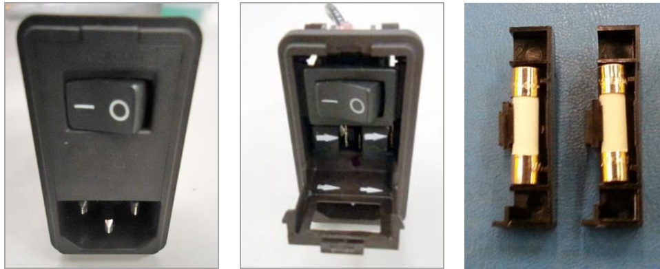
Figure 12. Replacing Fuses
